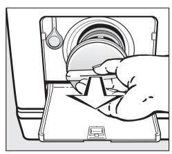
■ Remove the fluff filter completely.
